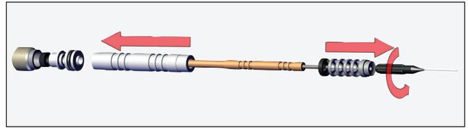
6. Prior to installation apply dielectric grease inside packing tube, completely full.
