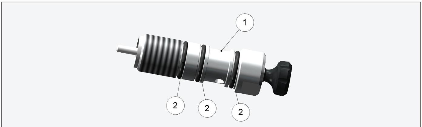
**REAR CARTRIDGE ASSEMBLY 80262-00 (ADJUSTABLE FLUID CONTROL)**
