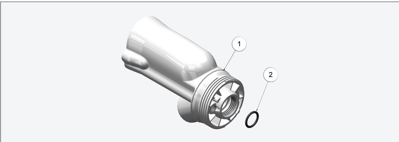
**RFXQ 65kV BARREL AND O-RING 80379-00**
