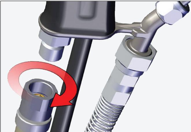
5. Trigger applicator with fluid off. Look for leaks in any connections
