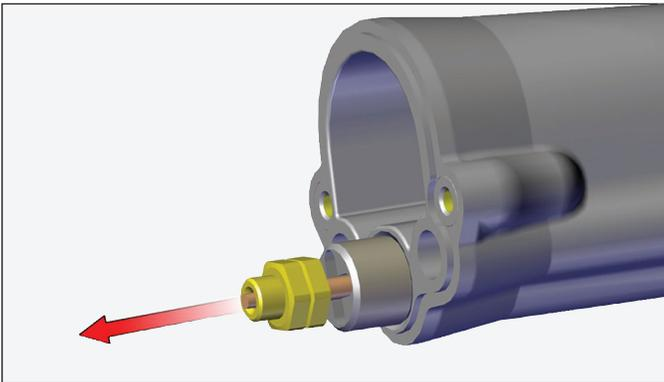
4. Remove jam nuts using 10mm wrench.
