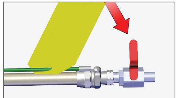
3. Discharge fluid into appropriate earth grounded metal container
