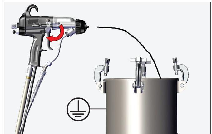
4. Load next color, solvent flush and/or remove applicator from installation as required.
