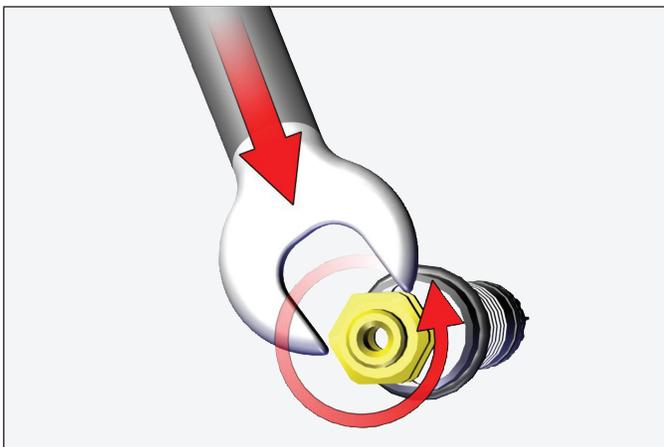
5. Remove all parts, clean with non-polar solvent. Inspect for any discolored areas. Replace parts as required.
