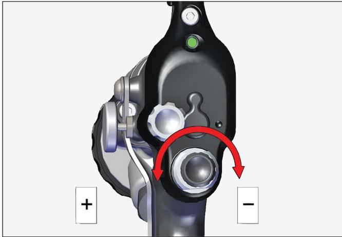
16. Adjust compensation valve with small driver.
