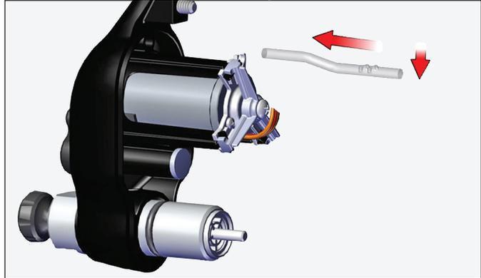
6. Install fluid valve cartridge.
