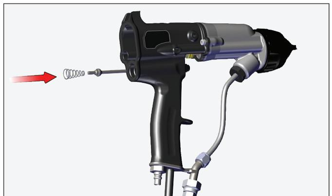
6. Tighten packing nut till light drag is felt on the shaft while moving it back and forth.
