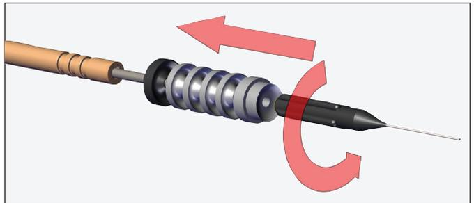
8. Insert packing tube onto shaft. Wipe excess grease over front parts and outside of packing tube.
