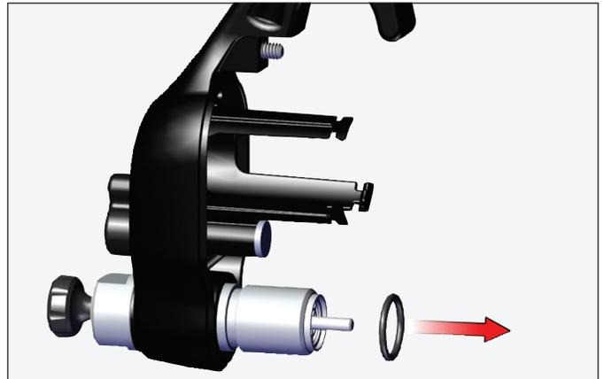
6. Push on edges to remove fluid valve cartridge.
