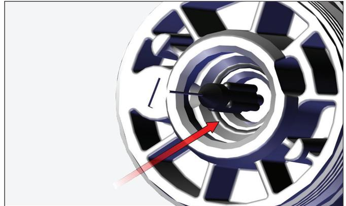
3. Install fluid nozzle using 80353-00 wrench. Tighten till nozzle seats on O-ring and then 1/8 additional turn.
