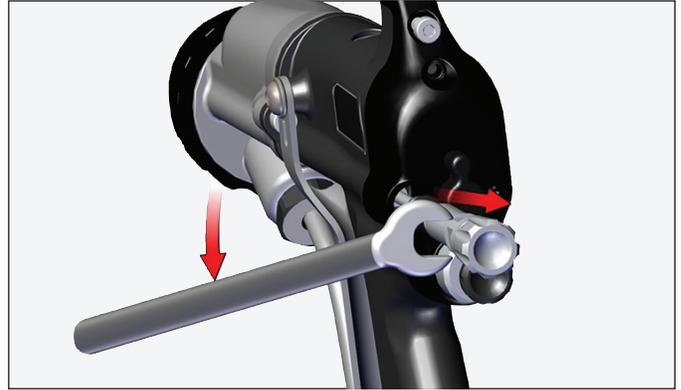
3. Remove rear cover and cartridge with 15mm wrench.
