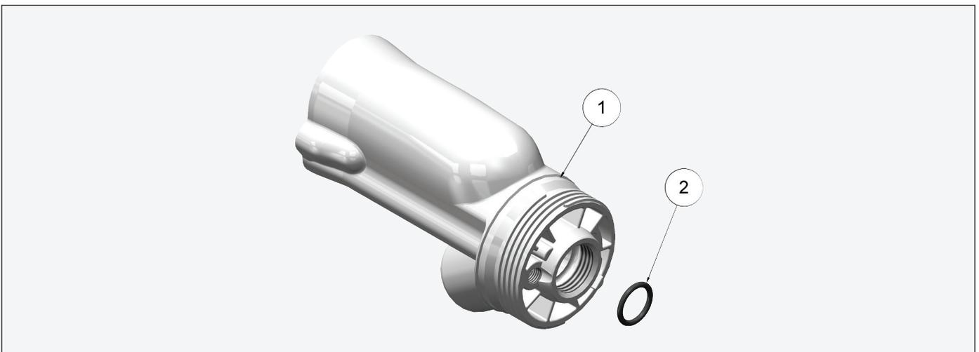
**RXQ 45kV BARREL AND O-RING 80376-00**
